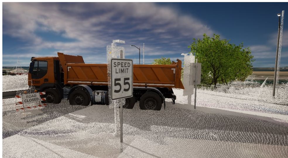
Figure 2. Example of how the point cloud was used as a guide for placing 3D static meshes (source: authors).
