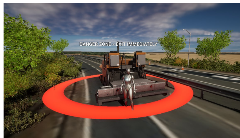
Figure 7. Simulated “danger zone” around an asphalt paver (source: authors).
