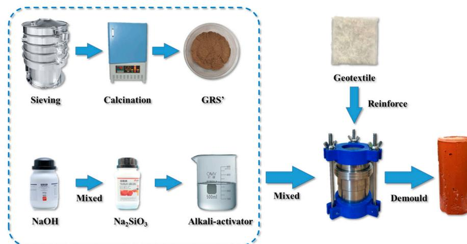
**Figure 3.** Sample preparation process.
