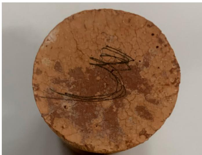
**Figure 13.** Cracks in D-W cycle samples.
