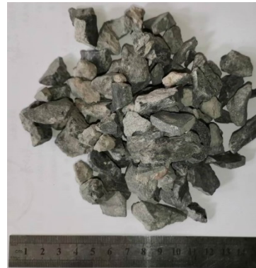
Figure 1. Coarse aggregates recovered from concrete after microwave heating, showing the composition and size distribution.
