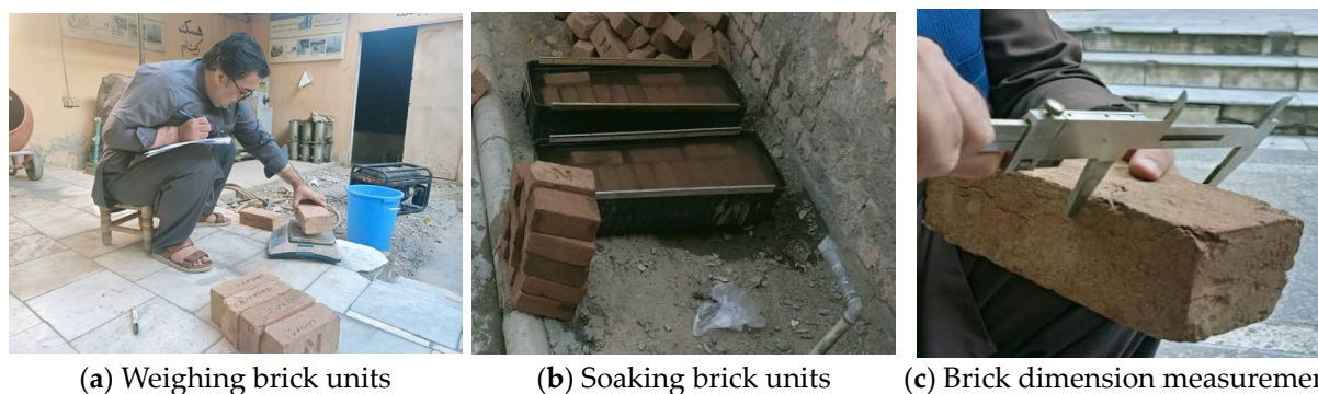
Figure 5. Brick preparation and measurement of physical properties.
