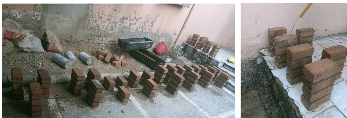
Figure 7. Masonry prism specimens during the curing stage.
