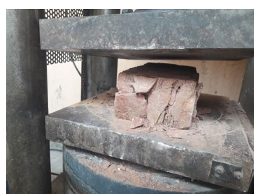
(a) Brick unit failure
