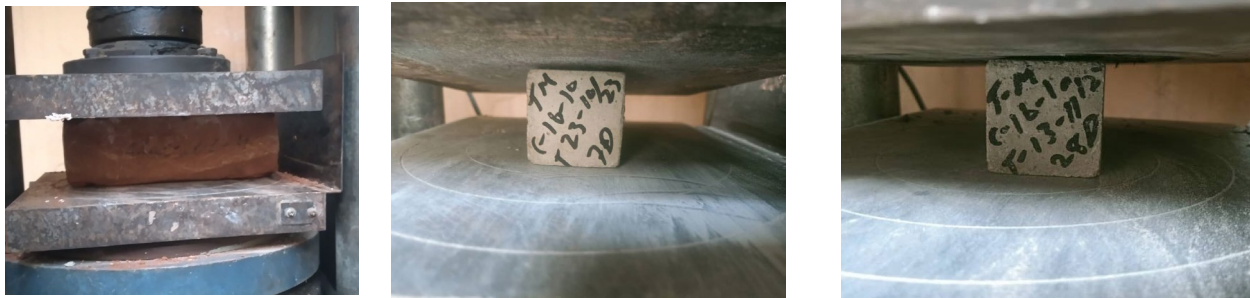
(a) Brick unit testing (b) Mortar cube testing on the 7th day (c) Mortar cube testing on the 28th day
