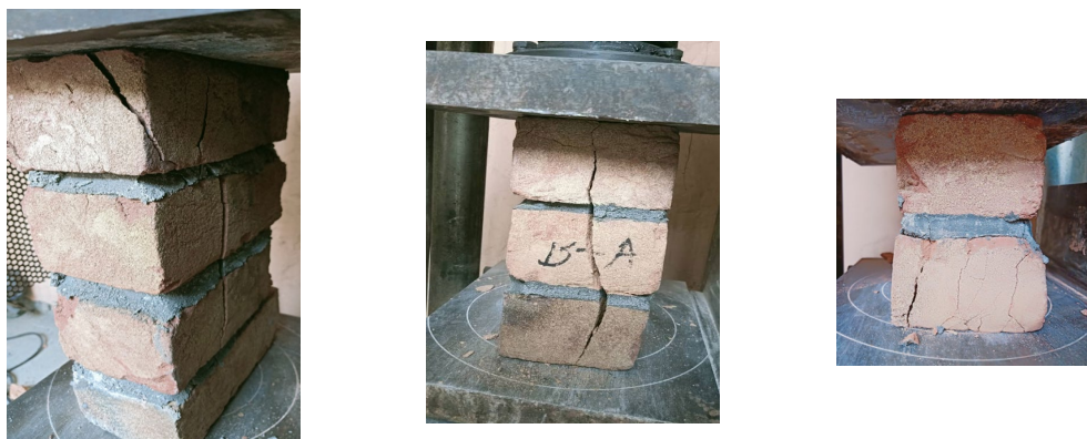
(a) Four brick layers of prism (b) Three brick layers of prism (c) Two brick layers of prism
