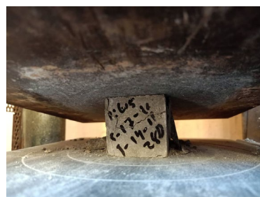
(b) Mortar cube failure after curing for 28 days
