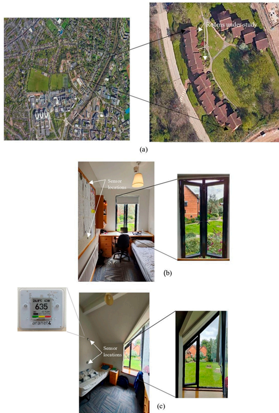
Figure 1. Study area: (a) location map, (b) photograph of Test 1 conducted in Room A, and (c) photograph showing the location of Tests 2, 3, and 4 carried out in Room B with a single window with a 20% allowable opening.
