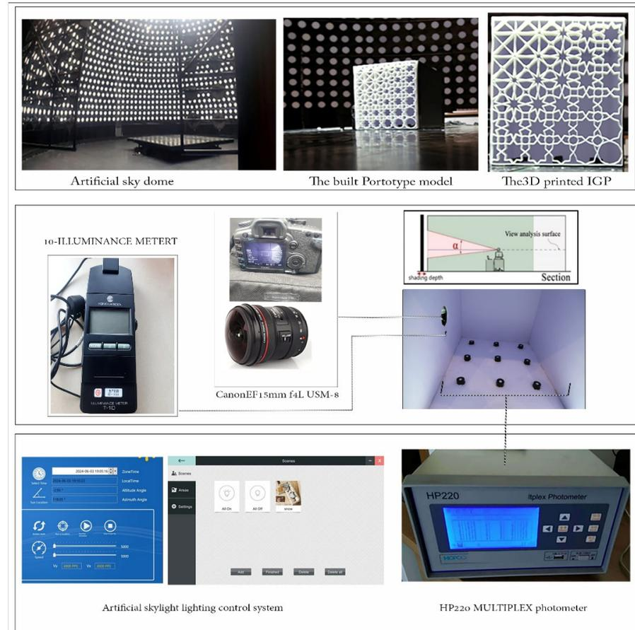
**Figure 8.** Experimental setup for the validation of the PSS shading system.
