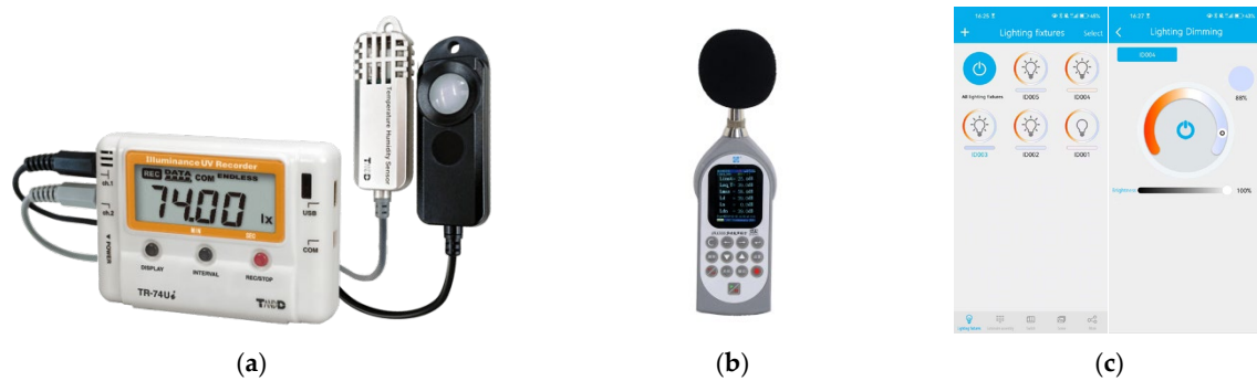
Figure 6. (a) Temperature, humidity, and illuminance recorder; (b) multi-function sound level meter; (c) illuminance and color temperature control terminals.
