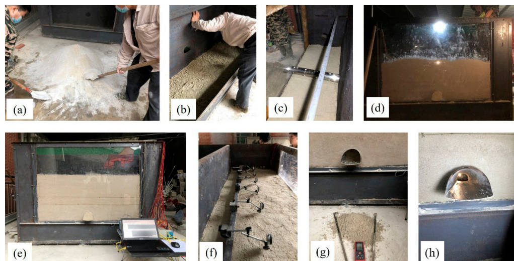
Figure 18. Model test processes: (a) Similarity materials production. (b) Materials filling. (c) Tunnels burying. (d) Continue filling. (e) Similarity materials curing. (f) Dial gauges arranging. (g) New tunnel excavation. (h) Excavation complete.
