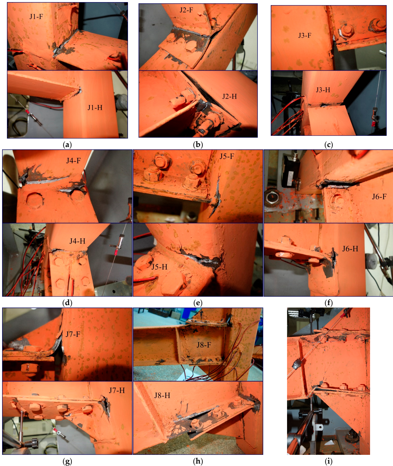
Figure 6. Failure modes of specimens: (a) J1-F & J1-H; (b) J2-F & J2-H; (c) J3-F & J3-H; (d) J4-F & J4-H; (e) J5-F & J5-H; (f) J6-F & J6-H; (g) J7-F & J7-H; (h) J8-F & J8-H; (i) J8-F.
