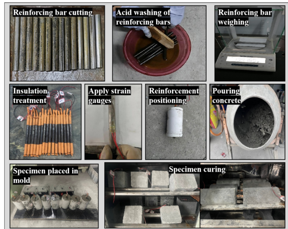
Figure 2. Reinforcement processing and specimen forming.
