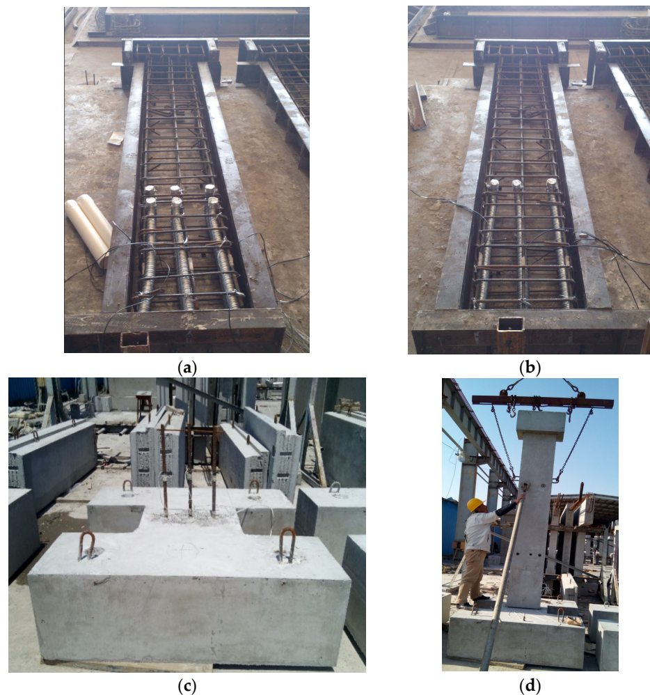
Figure 4. Specimen Fabrication Process: (a) Double-row Wall and Top Beam; (b) Single-row Wall and Top Beam; (c) Foundation Beam; (d) Assembly.
