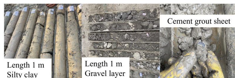
Figure 10. Soil core samples from the pile-side strata of the test piles.
