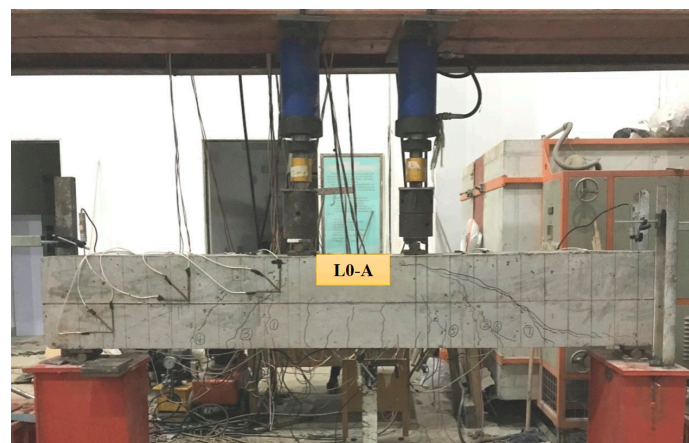
Figure 2. Test device, arrangements of SFRSCAC strain gauges and displacement meters.
