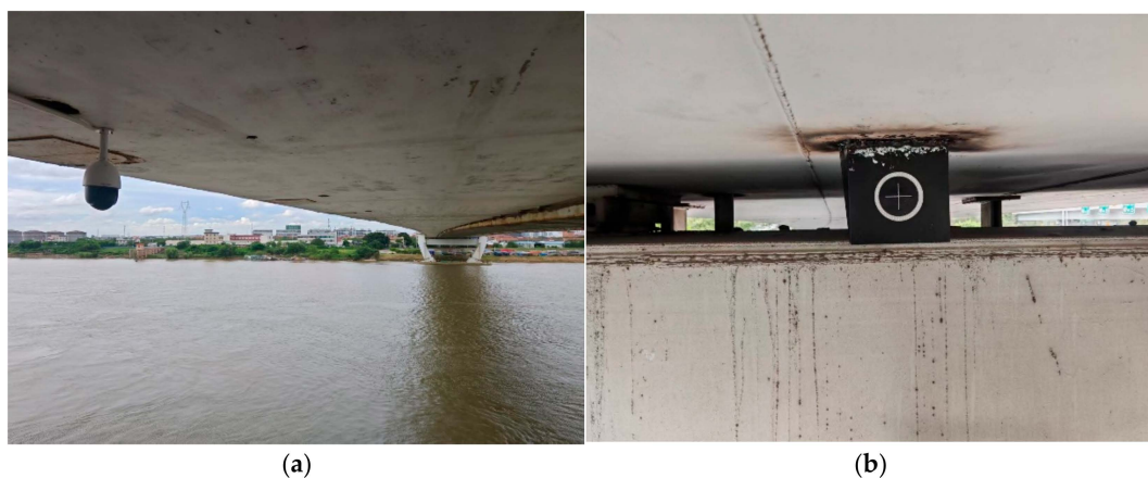
Figure 5. (a) Displacement measurement using a machine vision camera. (b) Machine vision target.
