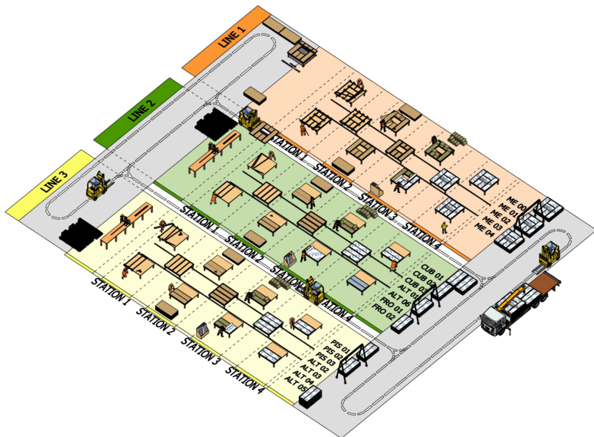
Figure 6. Simulated plant layout for production lines L1–L3 under the 18-operator configuration (6 per line). Source: authors.
