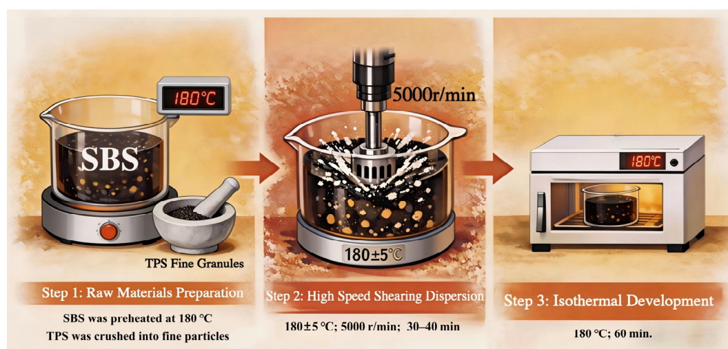
Figure 2. Preparation procedure for T&S modified asphalt.
