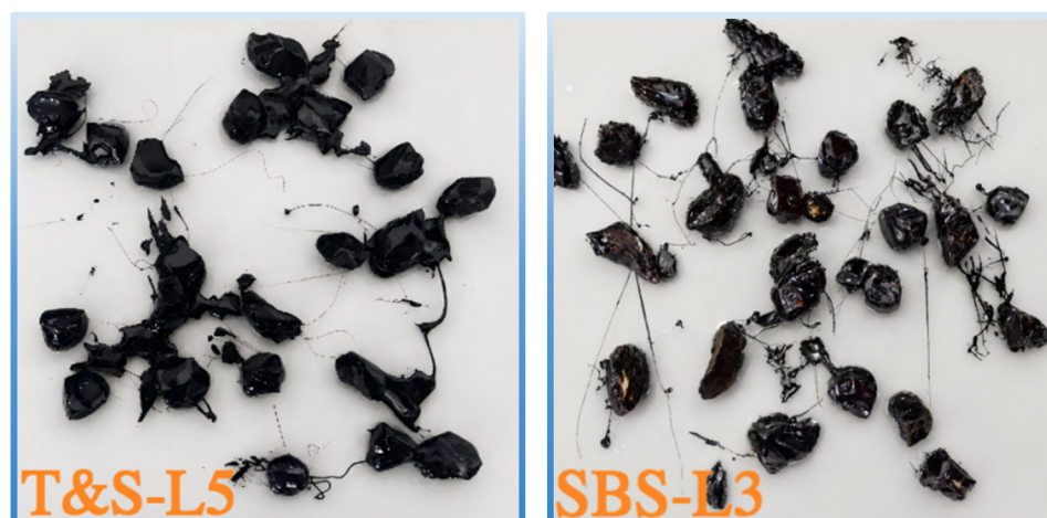
Figure 6. Asphalt adhesion evaluated by the water-immersion method.
