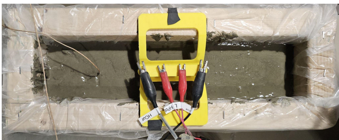
Figure 5. OPC paste experimental setup showing the four-electrode probe inserted into freshly mixed paste within the wooden formwork at the marked fill level (1.64 L).
