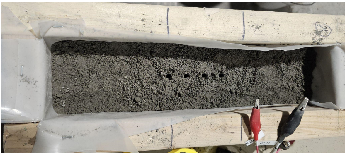
Figure 12. X-Hab 3D mixture at w/c = 0.45 showing granular, discontinuous microstructure insufficient for reliable electrical resistance measurement.
