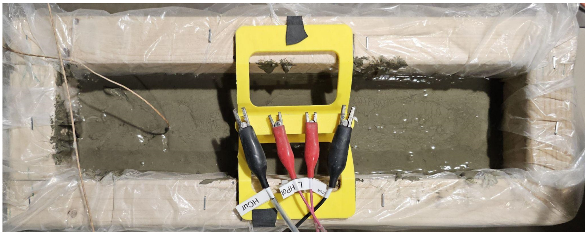
Figure 13. X-Hab 3D mixture at w/c = 0.51 showing cohesive, workable mortar with continuous microstructure suitable for reliable electrical resistance measurement.
