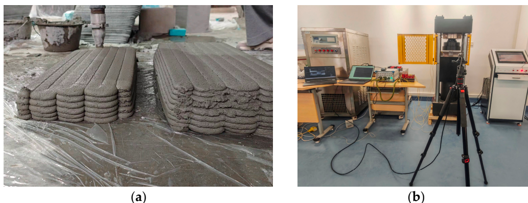
Figure 1. Experimental setup. (a) Gantry-type 3D concrete printer during the layer-wise deposition process. (b) DIC imaging configuration with high-resolution camera and speckle-patterned specimen mounted in the compression testing machine.
