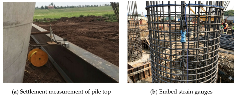
Figure 3. Settlement and axial force measurement device.
