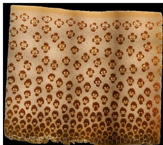
Figure 4. Enlarged image of Moso bamboo under 3D microscope.
