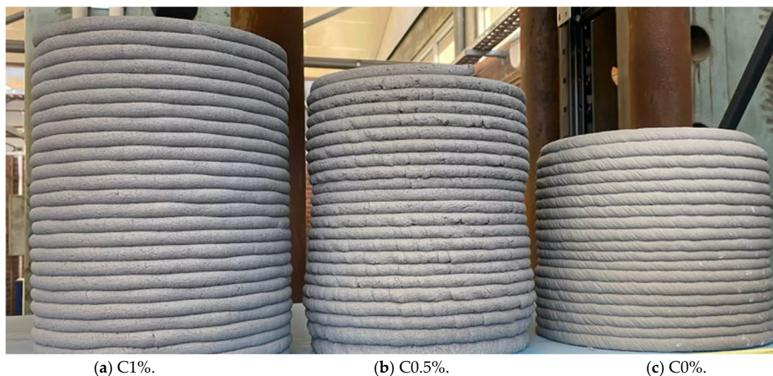
Figure 6. Representative printed cylindrical structures obtained during the buildability assessment.
