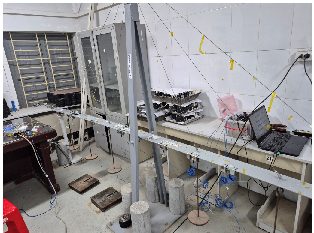
Figure 2. The cable-stayed bridge model utilized for data acquisition at the Bridge and Tunnel Department, University of Transportation and Communication (UTC), Hanoi, Vietnam.
