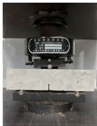
Figure 4. Fracture Toughness Test Setup.
