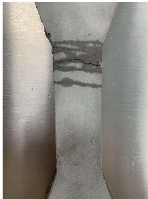
Figure 13. The photograph of the failed dog-bone specimens.
