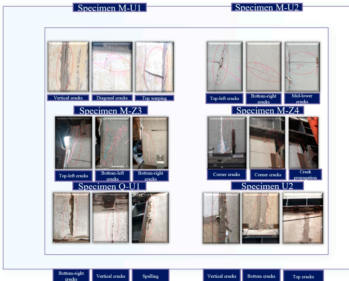
Figure 6. Observed failure patterns, showing extensive cracking and corner crushing in the U-type walls and localized corner cracking in the Z-type walls.
