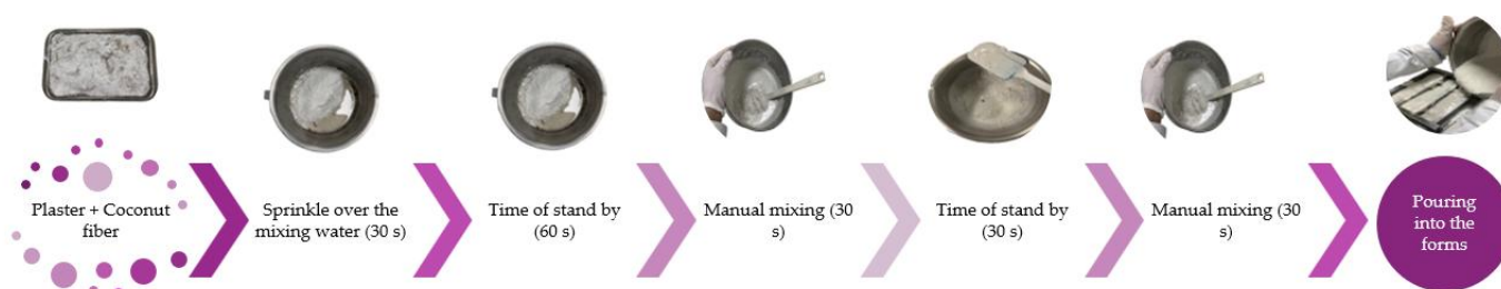
Figure 2. Procedure for preparing the composites.
