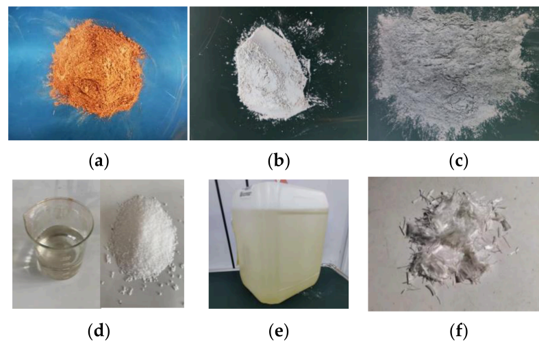
Figure 1. Test raw materials. (a) Bayer red mud; (b) ground granulated blast-furnace slag; (c) fly ash; (d) alkali activator; (e) foaming agent; (f) PVA fibers.
