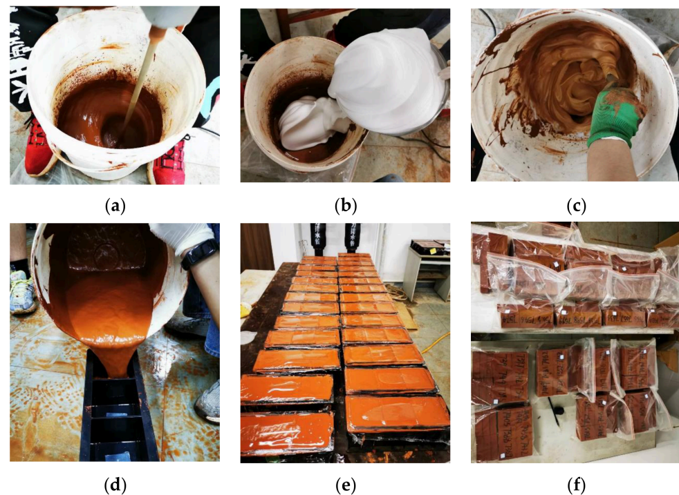
Figure 2. Preparation process of foam lightweight soil. (a) Stir the slurry mixture; (b) add foam; (c) stir the foam-based lightweight soil; (d) form the slurry into molds; (e) film-coating curing; (f) bagging care.
