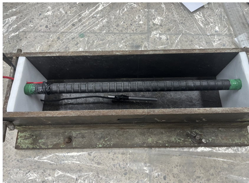
Figure 2. Example of a mold with reinforcing steel and a reference electrode pre-embedded prior to concrete casting.
