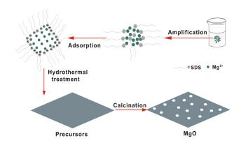
Scheme 1. Schematic illustration of the formation mechanism of SDS-assisted MgO nanosheets.
