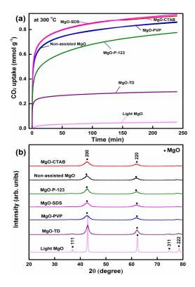
**Figure 1.** (a) The influence of different types of surfactants on the CO<sub>2</sub> capture capacity; (b) XRD spectra of MgO compounds with different types of surfactants.
