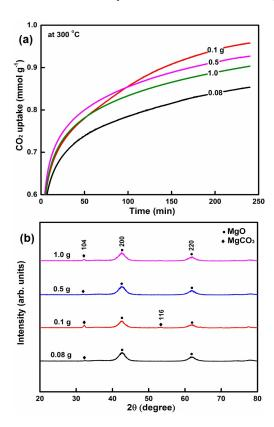
**Figure 3.** (a) The influence of SDS amount on the CO<sub>2</sub> capture capacity; (b) XRD spectra of MgO compounds with different amounts of SDS.
