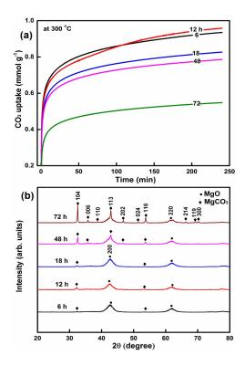
**Figure 4.** (a) The influence of reaction time on the  $CO_2$  capture capacity; (b) XRD spectra of MgO compounds at different reaction times.
