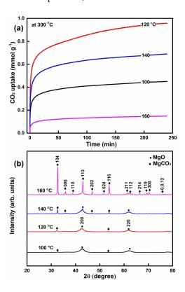
**Figure 5.** (a) The influence of reaction temperature on the  $CO_2$  capture capacity; (b) XRD spectra of MgO compounds at different reaction temperatures.
