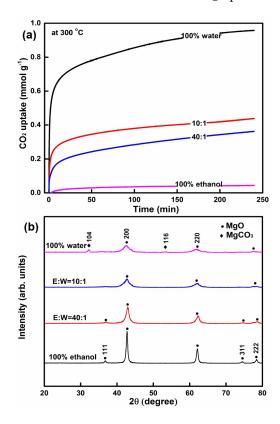
**Figure 2.** (a) The influence of ratios of ethanol and water on the CO<sub>2</sub> capture capacity; (b) XRD spectra of MgO compounds with different ratios of ethanol and water.
