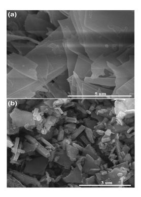
Figure 9. SEM images of (a,b) SDS-assisted MgO nanoparticles after adsorption/desorption for 20 cycles.
