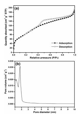
**Figure 6.** (a) Nitrogen adsorption-desorption isotherms and (b) pore size distributions of SDS-assisted MgO samples generated hydrothermally and calcined at 400 °C for 5 h.
