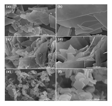
**Figure 7.** SEM images of (**a**,**b**) precursors; (**c**,**d**) MgO nanosheets after calcination at 400 °C for 5 h; (**e**,**f**) MgO-TC of different magnifications, respectively.
