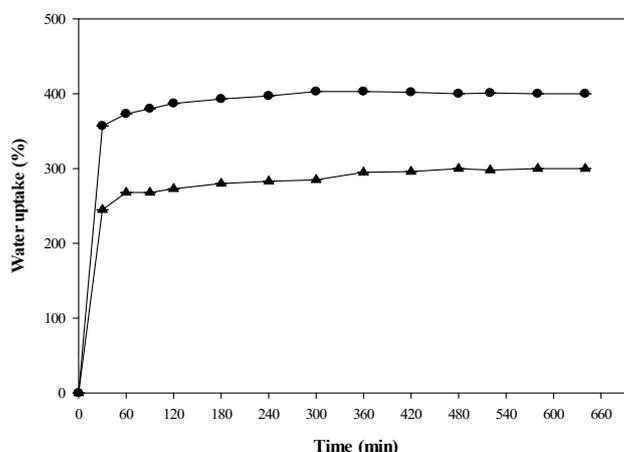
**Figure 1.** Swelling degree of hydrogels as a function of retention time: (▲) Gelatin-Alginate (GA), (●) Pectin-Alginate (PA).
