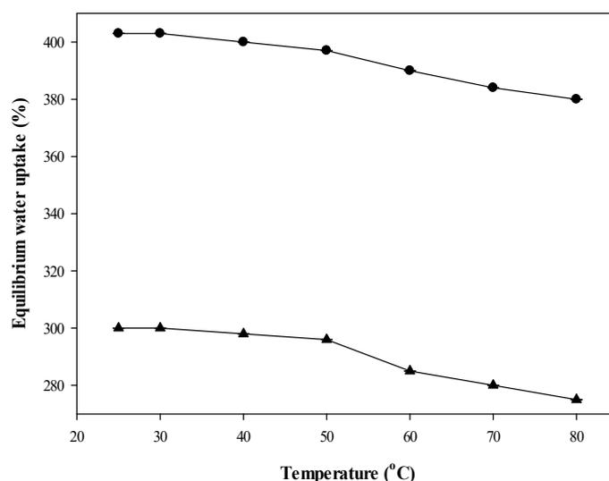
**Figure 2.** Swelling degree of hydrogels at different temperatures: (▲) Gelatin-Alginate, (●) Pectin-Alginate.
