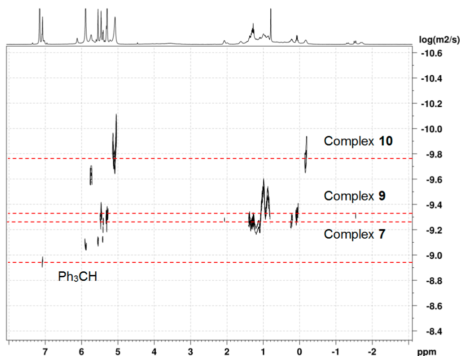
Figure 3. DOSY of the [\text{Cp}_2\text{ZrH}_2]_2\text{-ClAlEt}_2\text{-B}(\text{C}_6\text{F}_5)_3 (1:3:0.5) system in \text{C}_6\text{D}_6 ( T = 297.1\text{ K} ), heavy phase.
