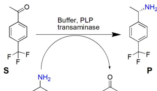
**Scheme 1.** Enzyme-catalyzed asymmetric transamination of 4'-(trifluoromethyl)acetophenone (S) with isopropylamine (IPA) as an amine donor to produce (*S*)-1-(4-trifluoromethylphenyl)ethylamine (P), and acetone (co-product).
