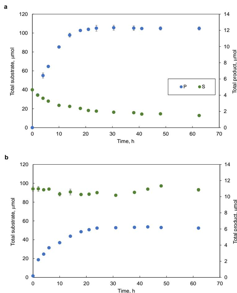
**Figure 3.** Quantities of 4'-(trifluoromethyl)acetophenone (S) consumed and of 4-trifluoromethylphenyl ethylamine (product; P) produced during the bioconversion catalyzed by TR<sub>8</sub> in one-phase (a), and two-phase (b) systems.
