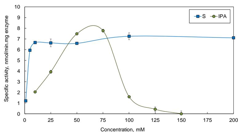
**Figure 1.** Effect of both isopropylamine (IPA) and 4'-(trifluoromethyl)acetophenone (S) concentrations on TR<sub>8</sub> activity.
