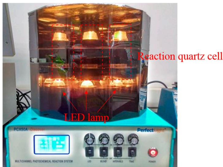
**Figure A1.** The image of a multichannel photochemical reaction system. A detailed description of the multichannel photochemical reaction system can be found in the following link. <https://www.perfectlight.com.cn/Product/detail/id/35.html> (visited on 09/05/2021).
