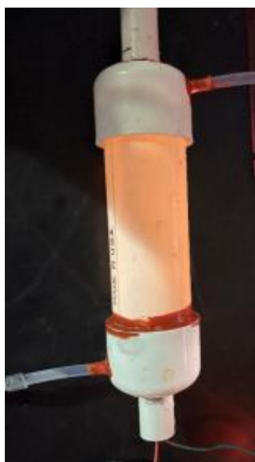
Figure 5. Photograph of one of four UV LED photocatalytic devices used in this study.
