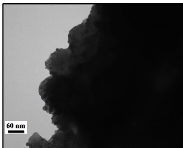
Figure 6. TEM image of SPION@CS-IL after the fifth run.
