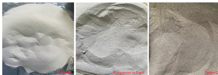
Figure 10. Physical appearance of fresh, regenerated, and spent catalysts.
