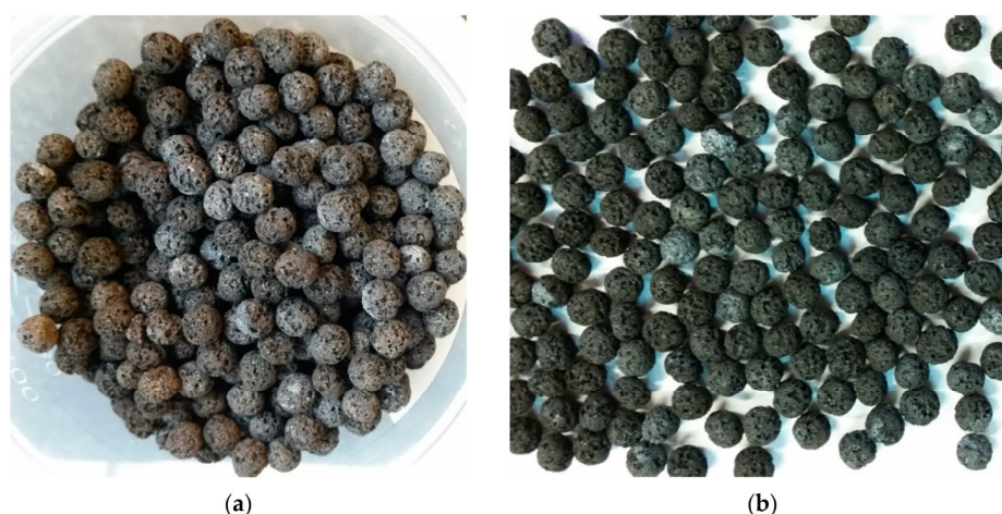
Figure 3. \text{MnO}_2 catalyst, supported on \alpha -alumina: (a) pre-test view and (b) post-test condition [86].
