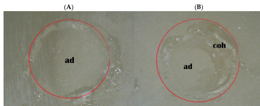
Figure 8. Stereomicroscopic micrographs of the Pi + Pi group: (A) adhesive failure and (B) mixed failure (ad, adhesive failure; coh, cohesive failure within the resin cement).
