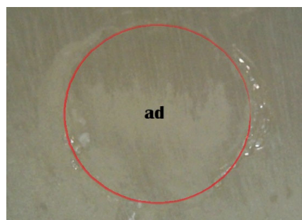
Figure 4. Stereomicroscope micrograph of control group (ad, adhesive failure).
