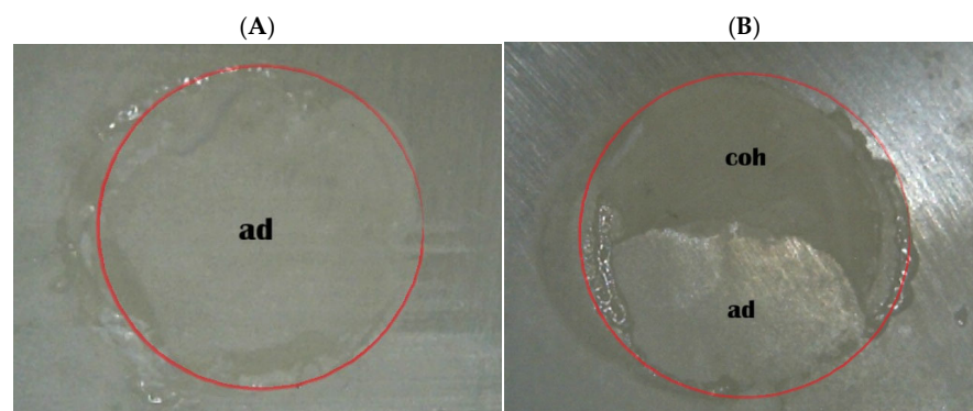
Figure 7. Stereomicroscopic micrographs of the SB + Pi group: (A) adhesive failure and (B) mixed failure (ad, adhesive failure; coh, cohesive failure within the resin cement).
