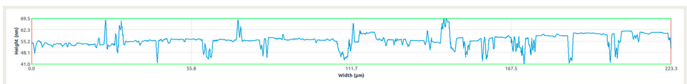
Figure 6. Surface profiling over a 223 \mu\text{m} long trace. The green lines indicate the maximum and minimum overall values for the test, the blue line indicates the profile at each measured point.
