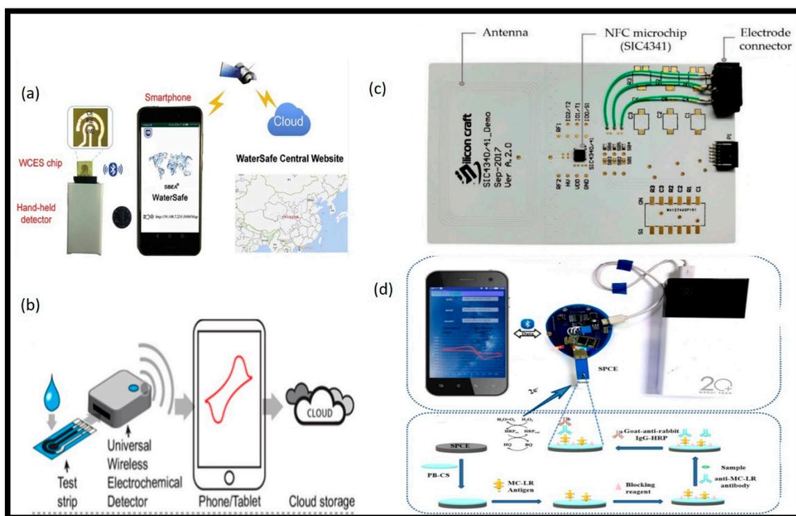
**Figure 3.** (a) Photograph of a smartphone-based water quality monitoring system, consisting of a WCES chip, a hand-held detector, a smartphone, and a WaterSafe central website [54]; (b) demonstration of how the UWED functions [55]; (c) hardware components consisting of a planar antenna, near-field communication (NFC) microchip, and connector for electrode interface [56]; (d) photograph of the SCEA showing the interface with MC-LR immunosensor and mobile power source [57].
