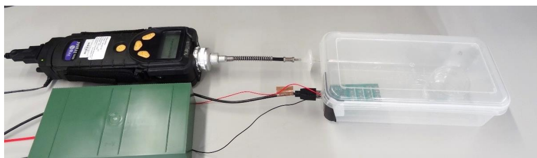
Figure 2. Measurement setup composed of a PID, the redundant power supply for the eNose, a transparent box containing the eNose, and a small glass plate to deposit the volatile in liquid form.
