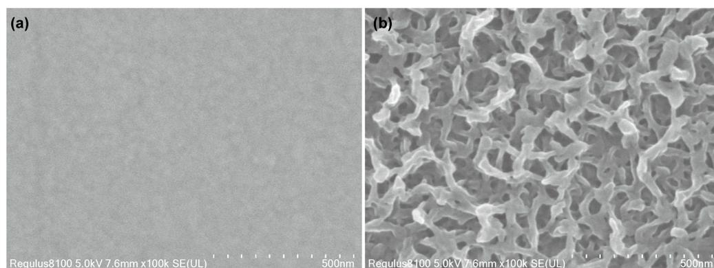
**Figure 5.** SEM images of (a) PEDOT:PSS film and (b) PEDOT:PSS/PEDOT (30 mC) film.
