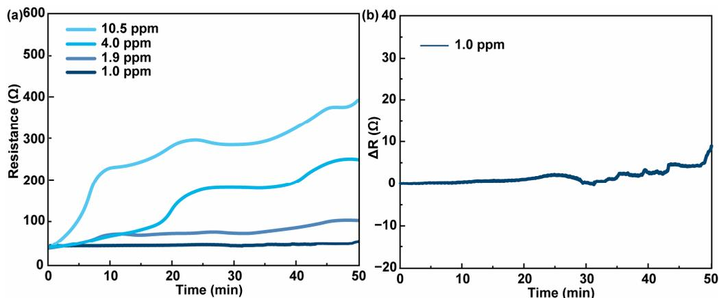
**Figure 8.** (a) Resistance-time curve of PEDOT film towards different concentrations of HPV and (b) resistance change-time curve of PEDOT film to 1.0 ppm HPV.
