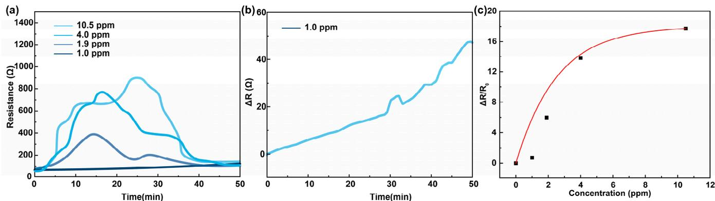
**Figure 7.** (a) Resistance-time curve to different concentrations of HPV, (b) resistance change-time curve to 1.0 ppm HPV and (c) resistance response-HPV concentration fitting curve of PEDOT:PSS/PEDOT (30 mC) film.
