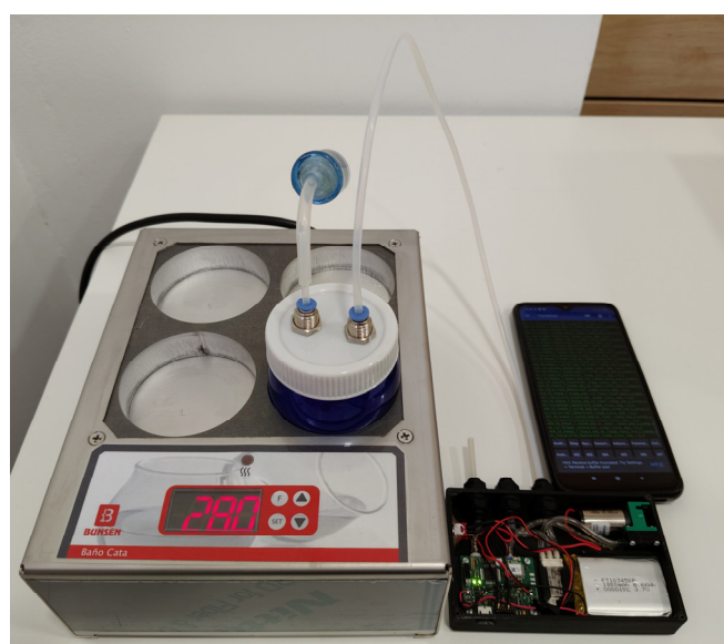
Figure 1. Prototype electronic nose equipped with MOS sensors.
