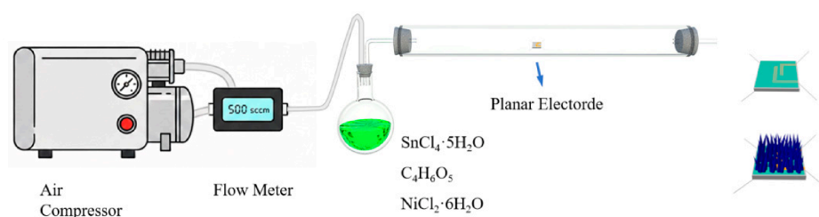
Figure 1. Schematic illustration of the preparation of Ni-SnO 2 films via the AACVD.
