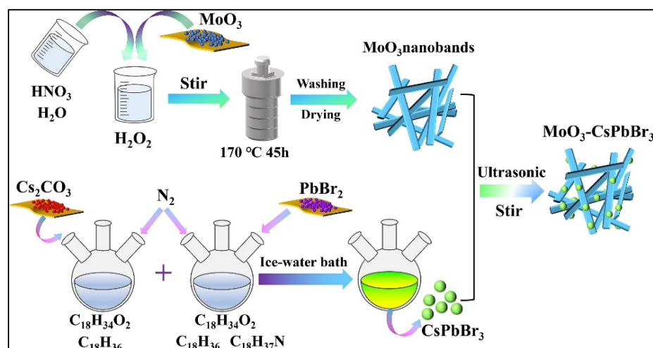
Figure 11. Schematic illustration of the preparation of \text{MoO}_3 and \text{MoO}_3\text{-CsPbBr}_3 composite. Reproduced with permission [145].
