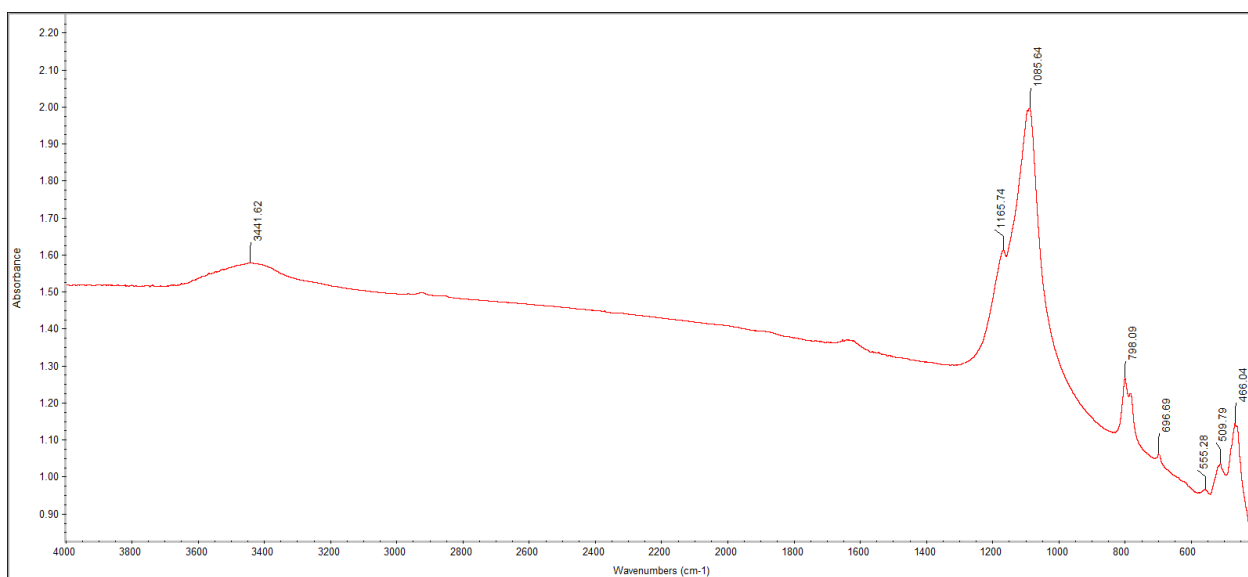
Figure 1. FTIR spectroscopy of TRIBALLOY® T-800 with TiC.
