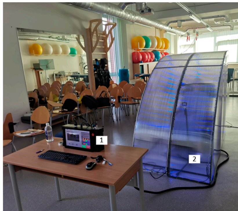
Figure 4. An overview of the entire system in real operating conditions: 1—control computer, 2—relaxation system with a chair inside.
