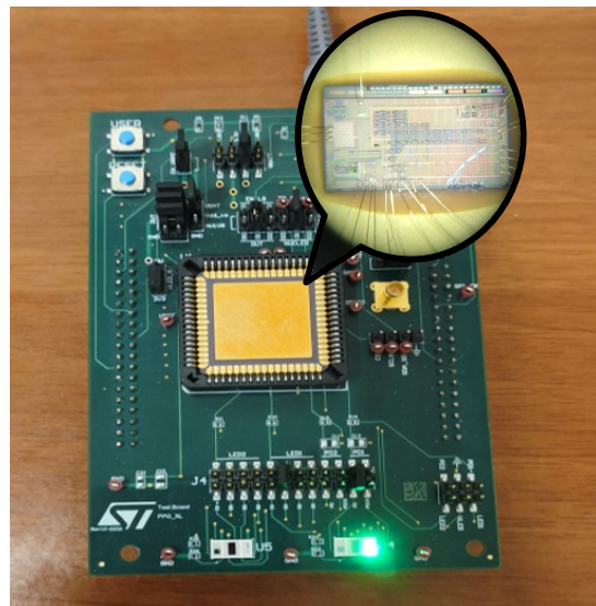
Figure 9. PPG sensor ASIC mounted on the application board.
