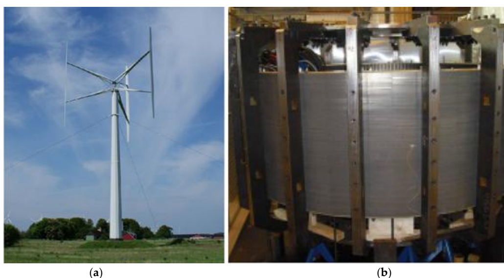
Figure 13. (a) Vertical Wind 200 kW (b) Synchronous generator for H-rotors. [56]
