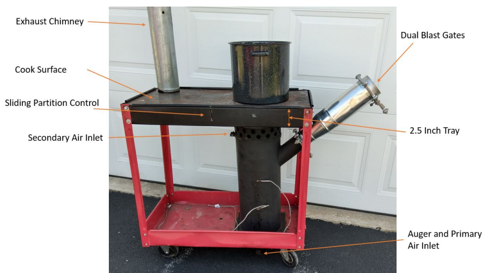
Figure 4. Fabricated cookstove on mobile cart that can be transported to testing location. The single pot indicates a one-hole cooksurface used for water boiling tests (described below).
