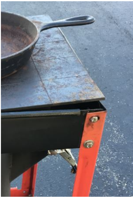
Figure 13. Warping of cookstove cooksurface due to temperature differences.
