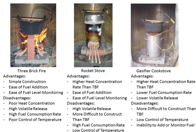
Figure 1. Comparison of cooking methods from [3,8,9].
