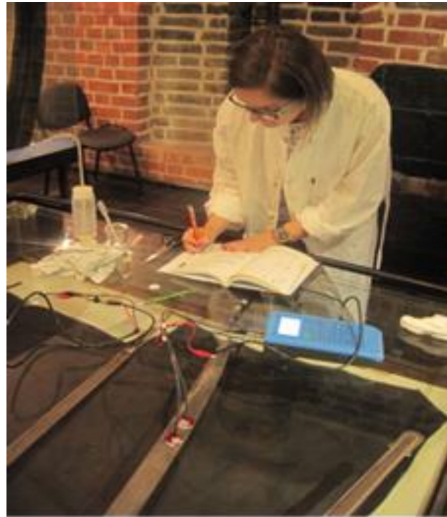
Figure 9. ENM testing on a non-commissioned officer sword of the Russian Navy, worn between 1871–1894.
